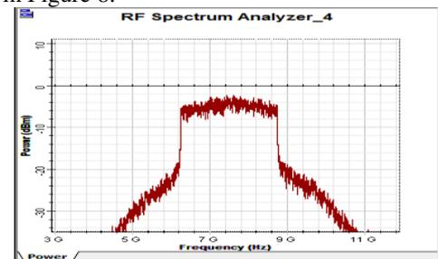
Figure8. RF Signal after BPF
