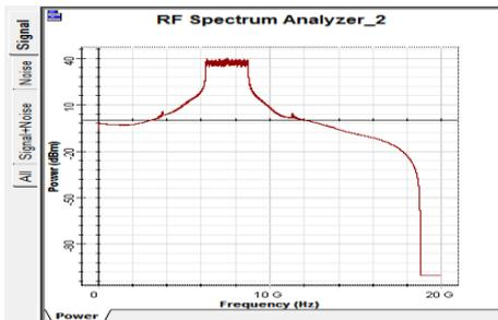
Figure5. OFDM Signal in the Frequency Domain
