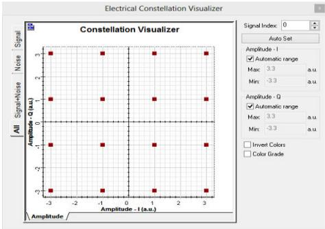
Figure3. 16 QAM Encoder Constellation Diagram
