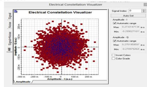
Figure9 Constellation Diagram of the 10 G bits/s One Users DD-OFDM at the Receiver Side after SMF of 100 km
