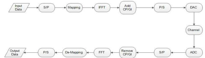
Figure 2. OFDM Block Diagram
