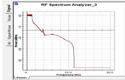
Figure4. Filtered OFDM signal by LP filter
